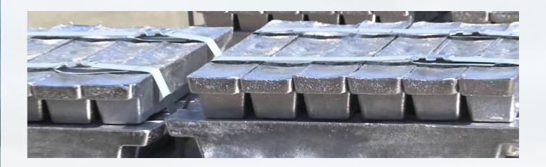
Aluminum ingot for remelting is produced by molten salt electrolysis method using alumina.
